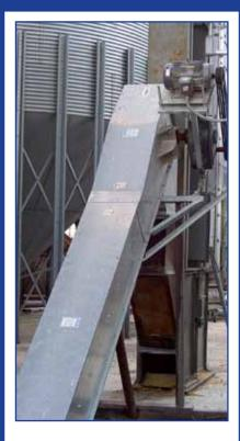
Horizontal and Incline Drag Conveyors
